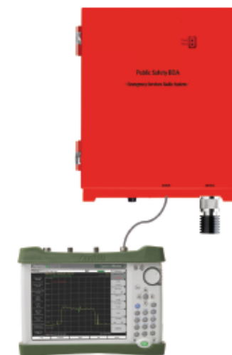
Figure 22.12.1 Measuring UL Noise Power from BDA
