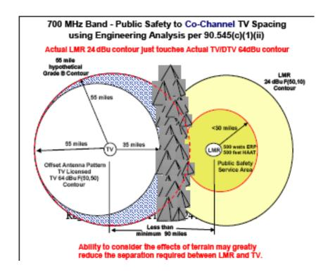
4.5 Note that 200 ft AGL limitations on 700 MHz control stations is much higher than the 100 ft AGL limitation used at UHF. Limiting control station antenna height and/or ERP may greatly reduce land mobile to TV contour spacing.
