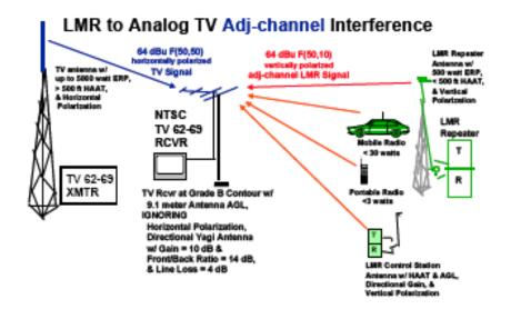
The equivalent ratios for a DTV station's 41 dB F(50,90) desired field strength contour are land mobile 17 dB F(50,10) contour for co-channel and land mobile - 23 dB F(50,10) contour for adjacent channel.
